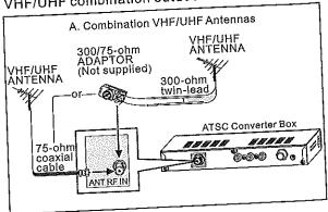
Using separate VHF and UHF outdoor antenna.
