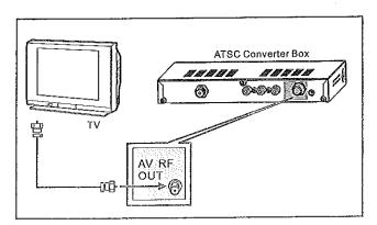
Note: RF output is modulated with current channel audio.
