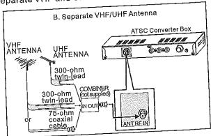
Connect an outdoor antenna cable lead-in to F-Type terminal. (Notice: F-Type connector should be finger-tightened only.)
