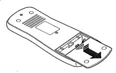
2 Install two AA batteries making sure the polarity (+ / -) is correct.
