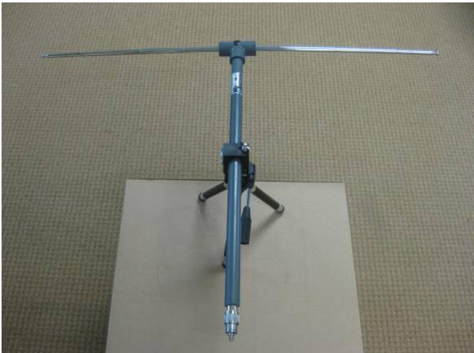
Figure 12. Reference dipole
