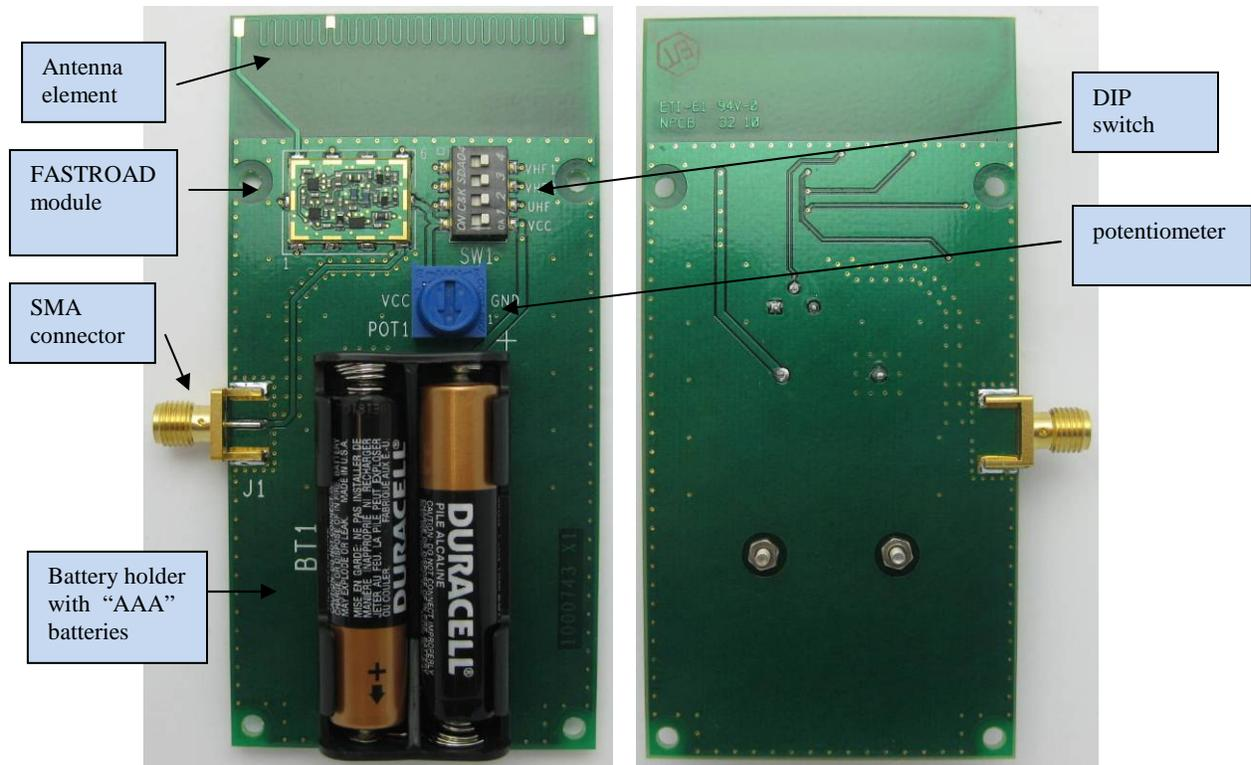
Figure 5. Demonstration board containing FASTROAD prototype active, tunable module; top (left) and bottom (right) sides of the demonstration board are shown
