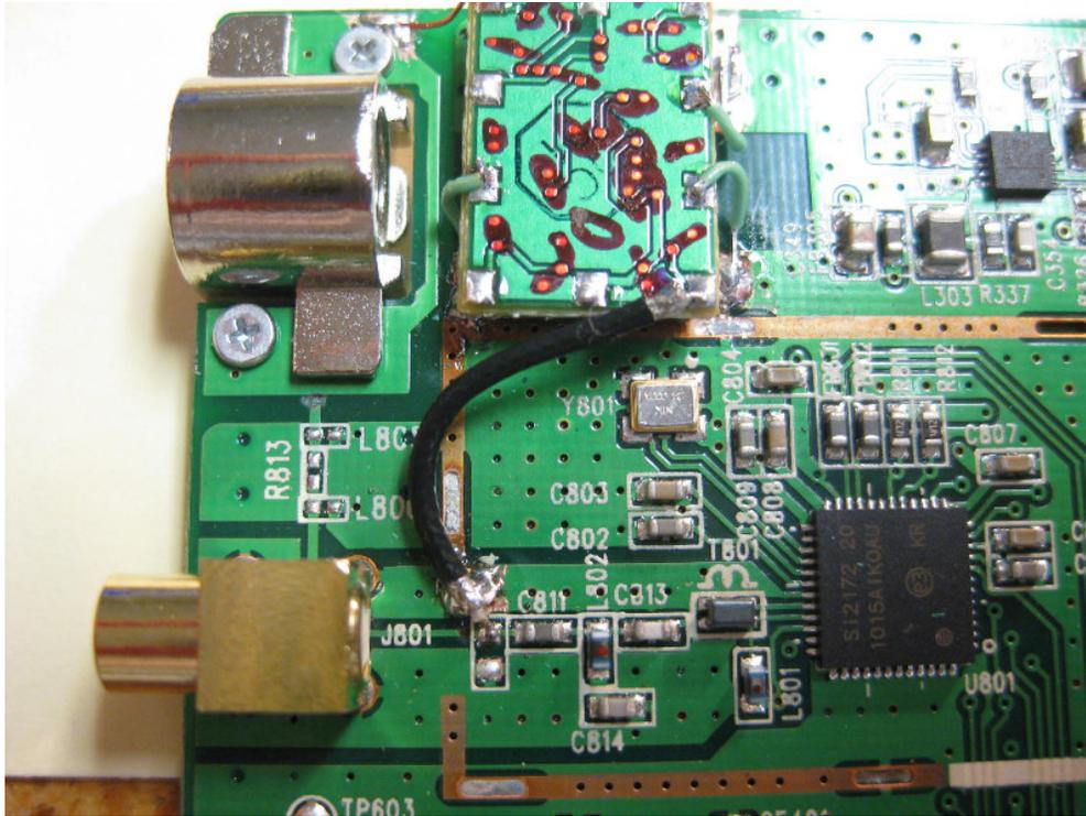
Figure 25. FASTROAD ATM installed in TV
