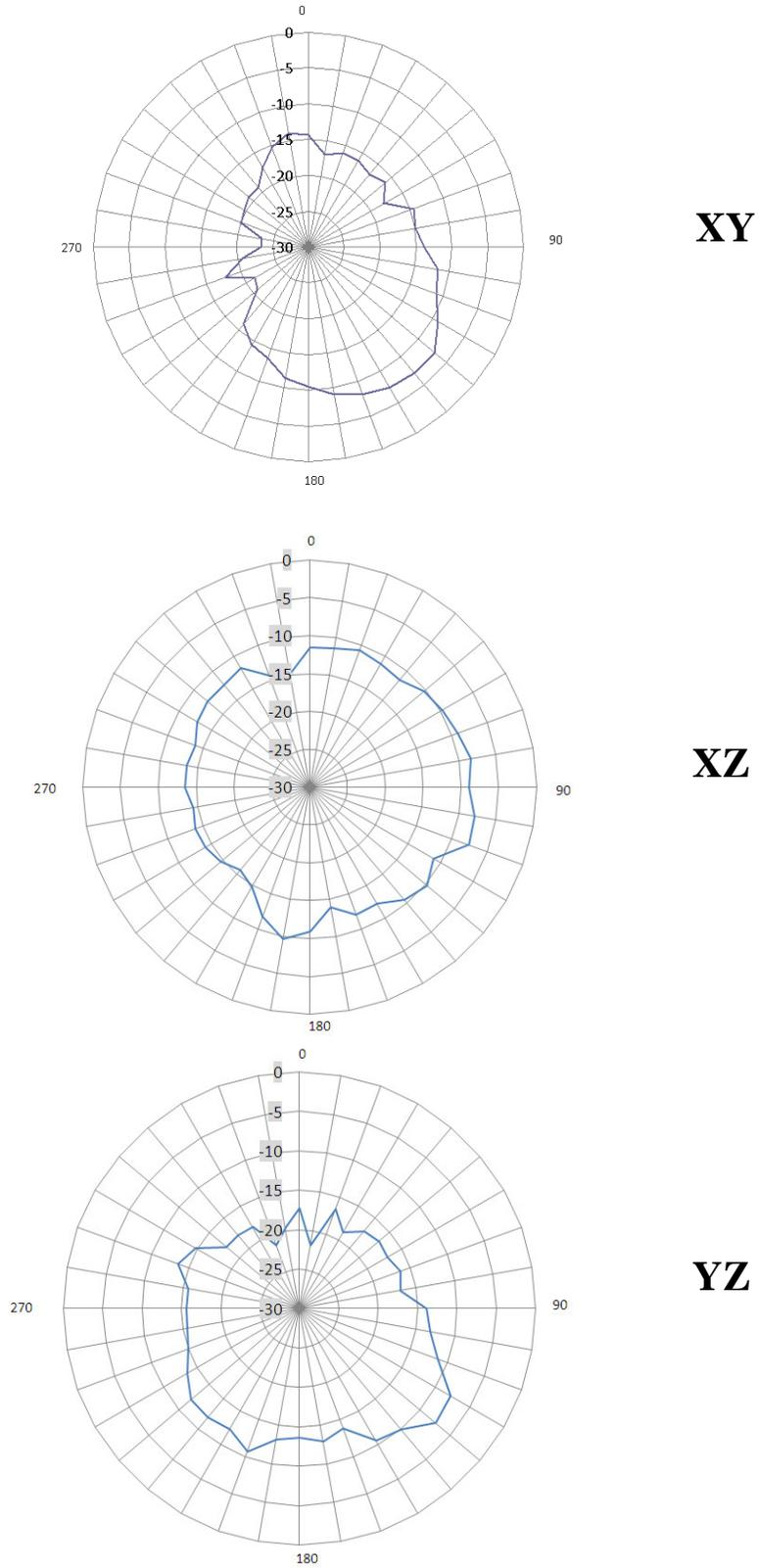
Figure 39. 2D radiation patterns at 105 MHz; scale is in dBi
