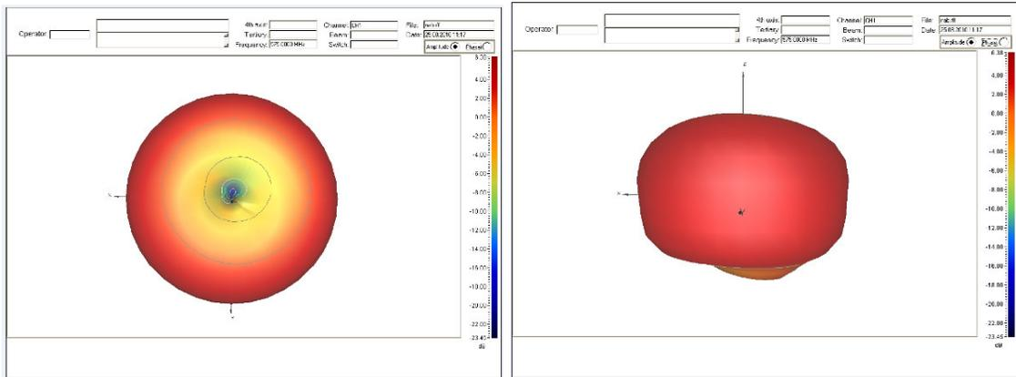
Figure 44. 3D radiation pattern at 585 MHz
