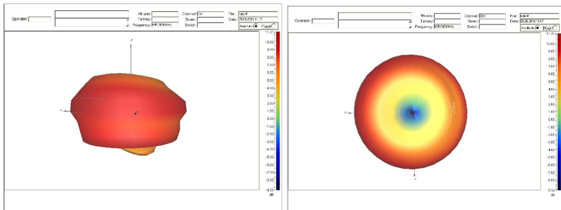
Figure 45. 3D radiation pattern at 695 MHz
