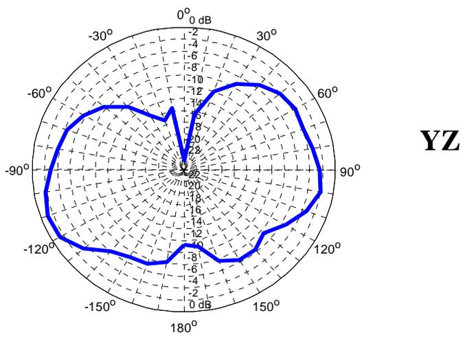
Figure 46. 2D radiation patterns at 470 MHz; scale is in dBi
