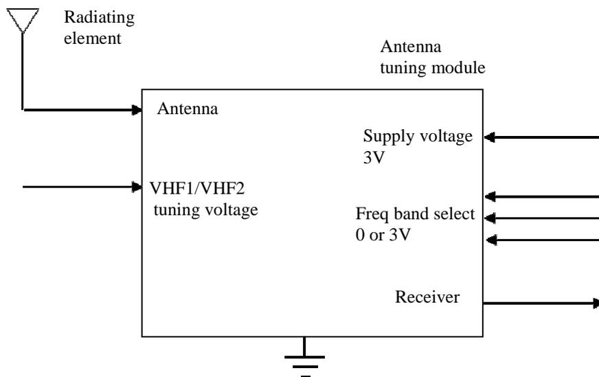
Figure 2. NAB FASTROAD embedded antenna control schematic
