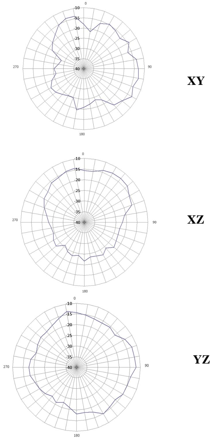
Figure 37. 2D radiation patterns at 89 MHz; scale is in dBi
