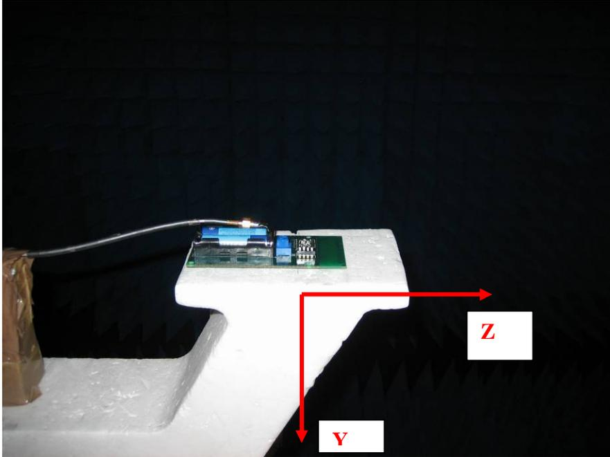
Figure 16. FASTROAD demonstration board mounted in anechoic chamber
