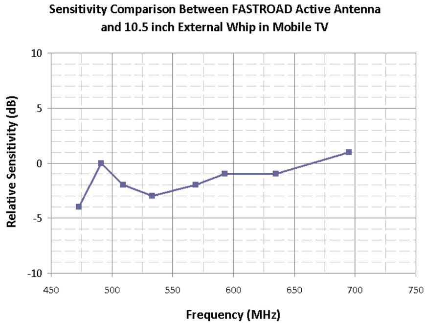
Figure 36. Measured comparison receiver sensitivity at UHF
