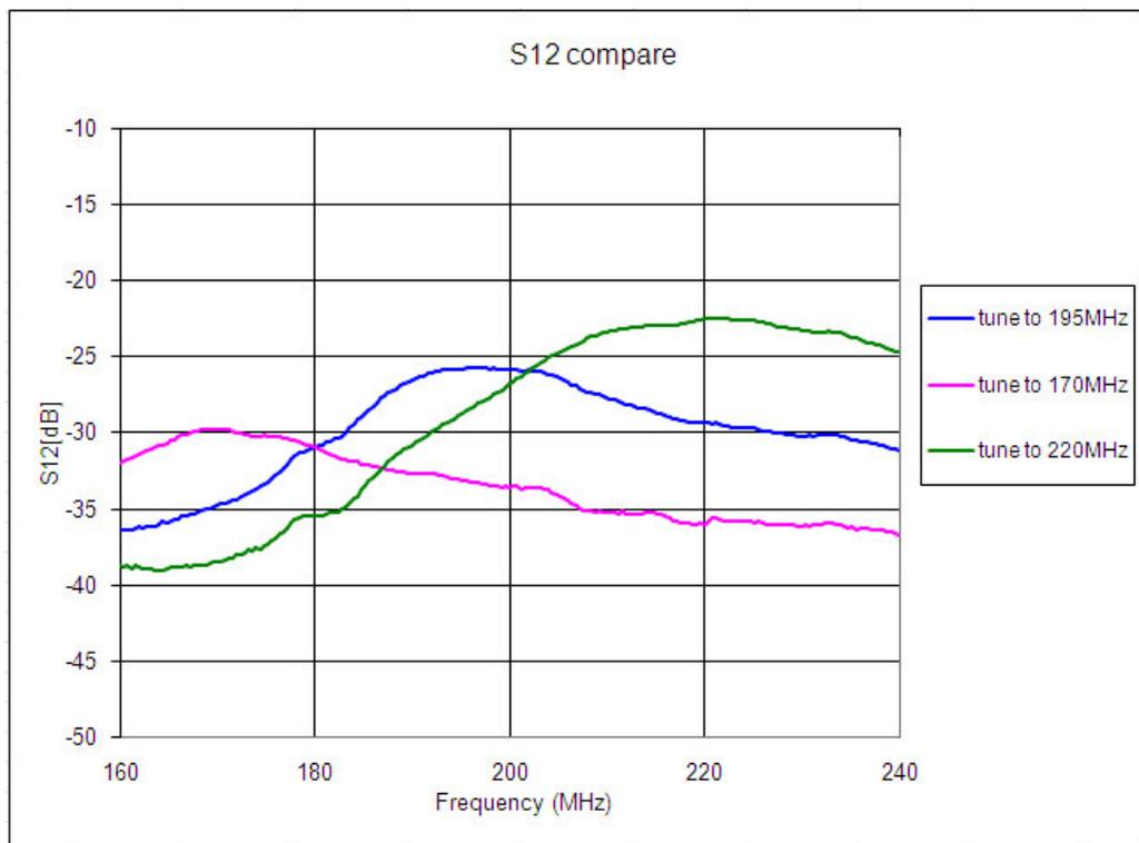
Figure 8. Tuning data for the VHF2 tuning circuit in the FASTROAD module
