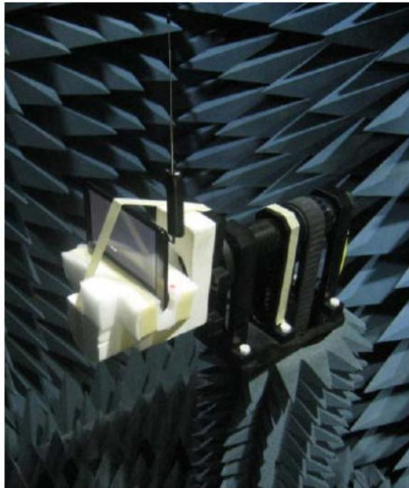
Figure 30. Baseline mobile TV in anechoic Chamber during test
