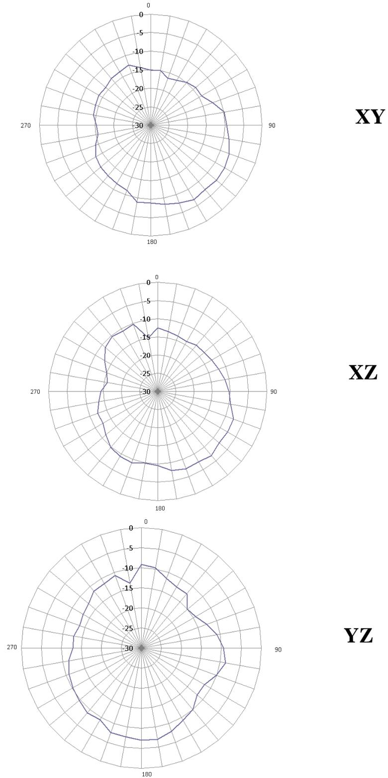
Figure 41. 2D radiation patterns at 183 MHz; scale is in dBi
