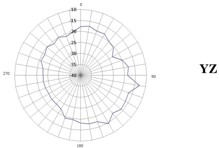
Figure 40. 2D radiation patterns at 175 MHz; scale is in dBi
