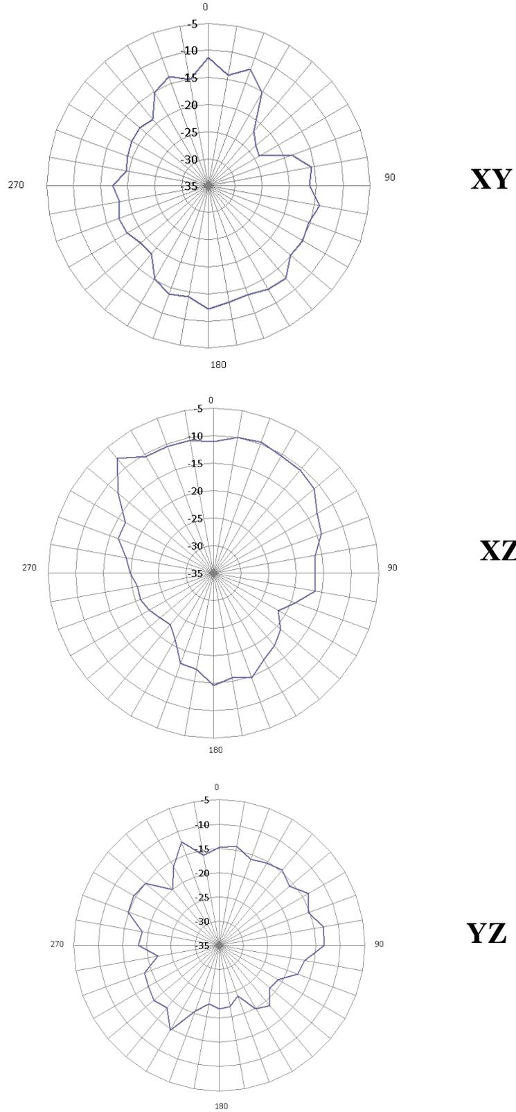
Figure 38. 2D radiation patterns at 96 MHz; scale is in dBi
