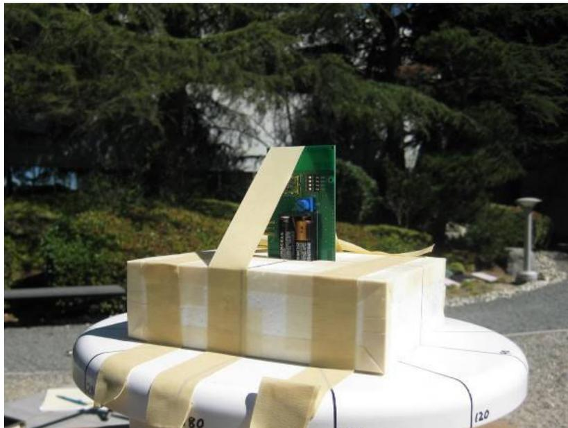
Figure 10. Antenna under test on turntable
