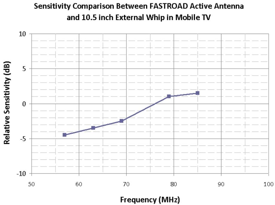
Figure 34. Measured comparison receiver sensitivity at VHF1
