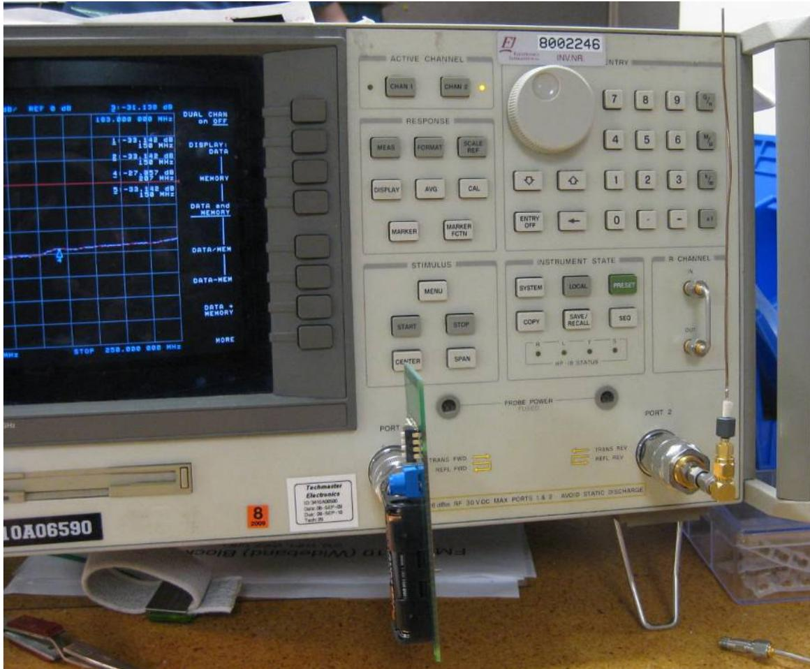
Figure 6. Demonstration board containing the FASTROAD module and antenna element connected to a network analyzer
