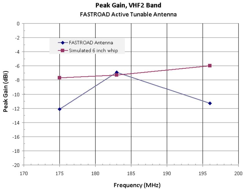
Figure 19. Measured peak gain of FASTROAD active tunable antenna at VHF2 band compared to simulated peak gain of 6 inch external whip antenna
