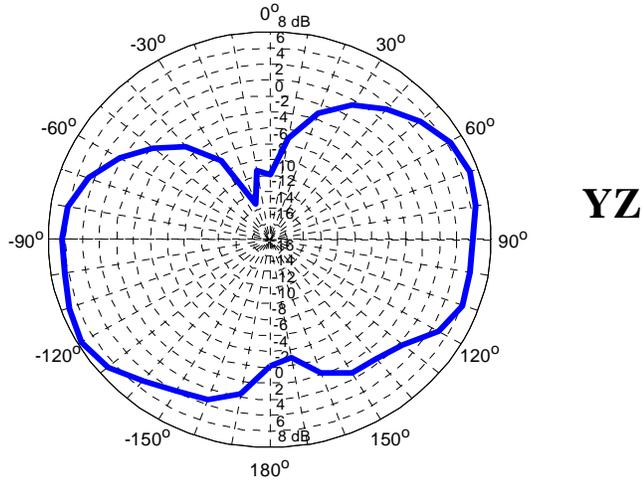
Figure 47. 2D radiation patterns at 585 MHz; scale is in dBi
