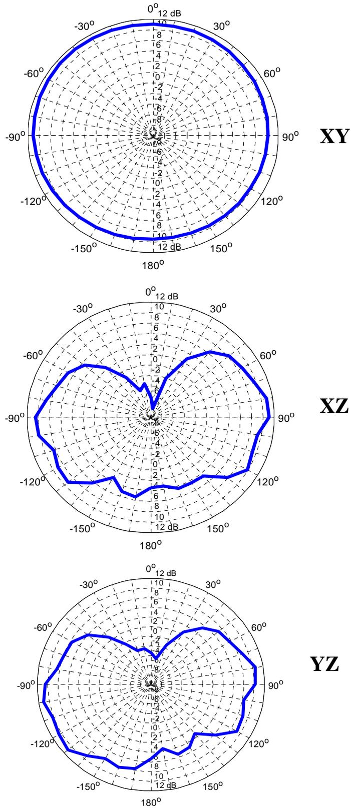
Figure 48. 2D radiation patterns at 695 MHz; scale is in dBi
