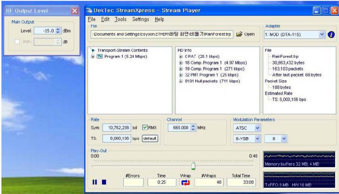
Figure 29. Screen shot of program used to control ATSC transmitter
