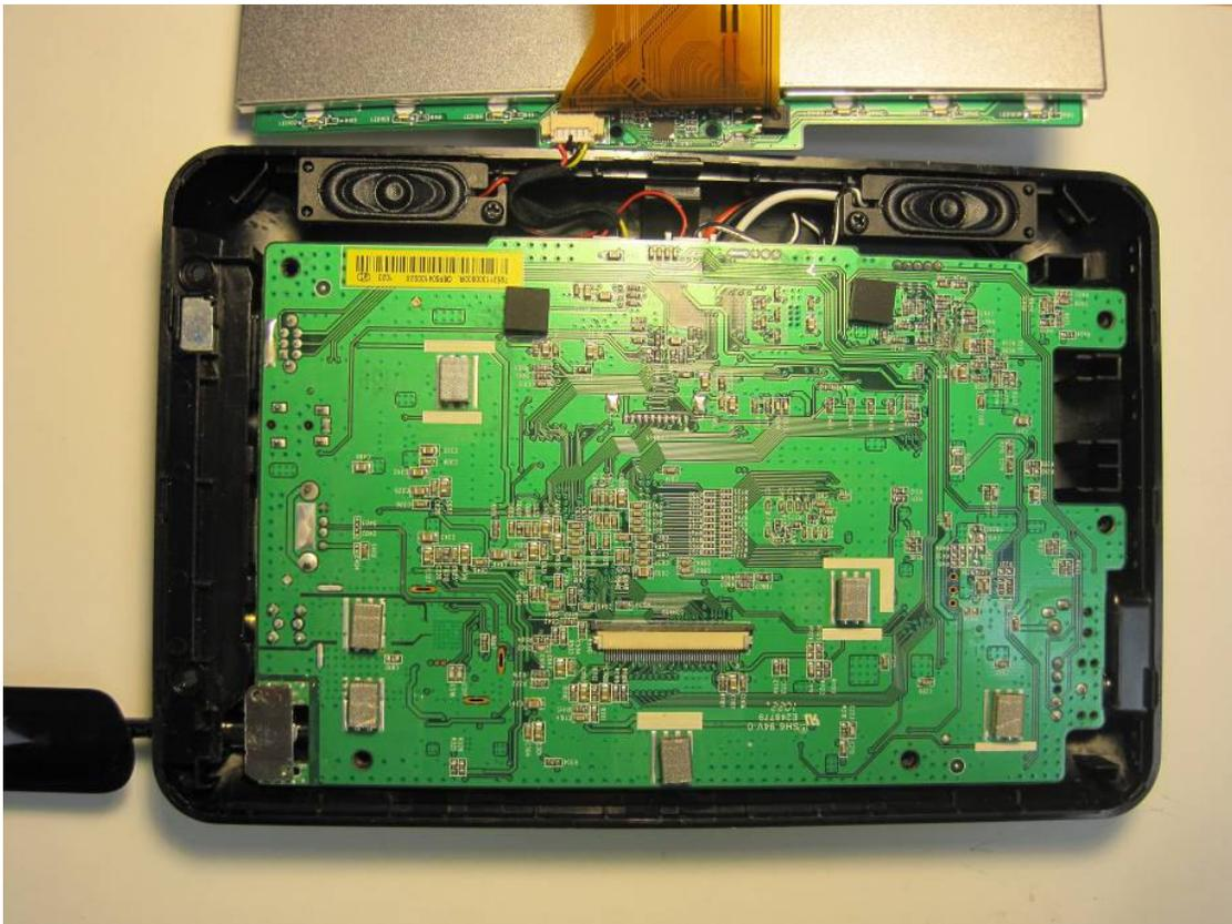
Figure 24. Mobile TV circuit board prior to modification
