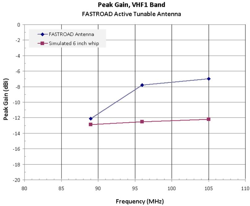
Figure 18. Measured peak gain of FASTROAD active tunable antenna at VHF1 band compared to simulated peak gain of 6 inch external whip antenna
