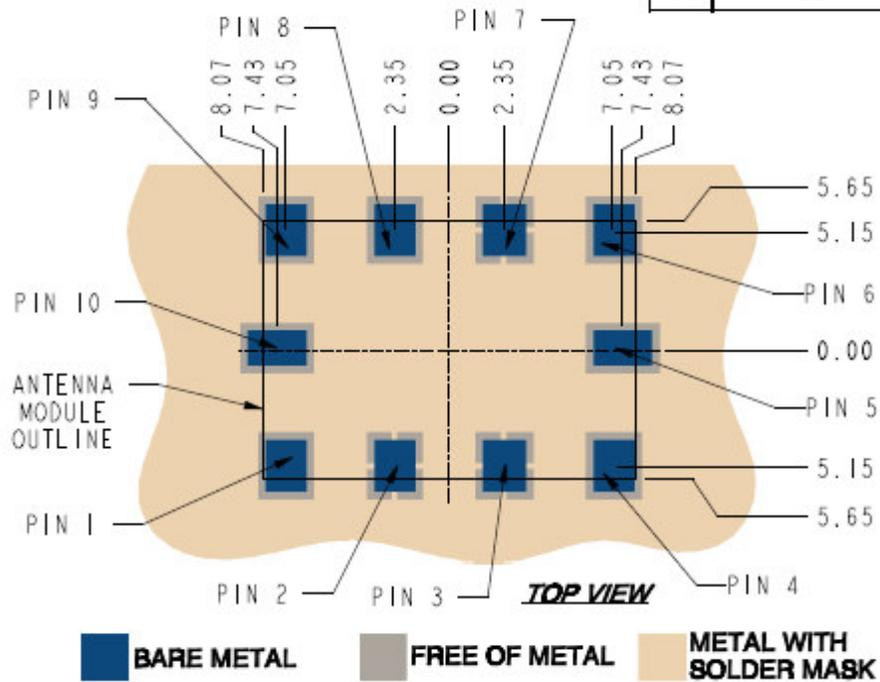
Figure 23. PCB pad layout for FASTROAD ATM
