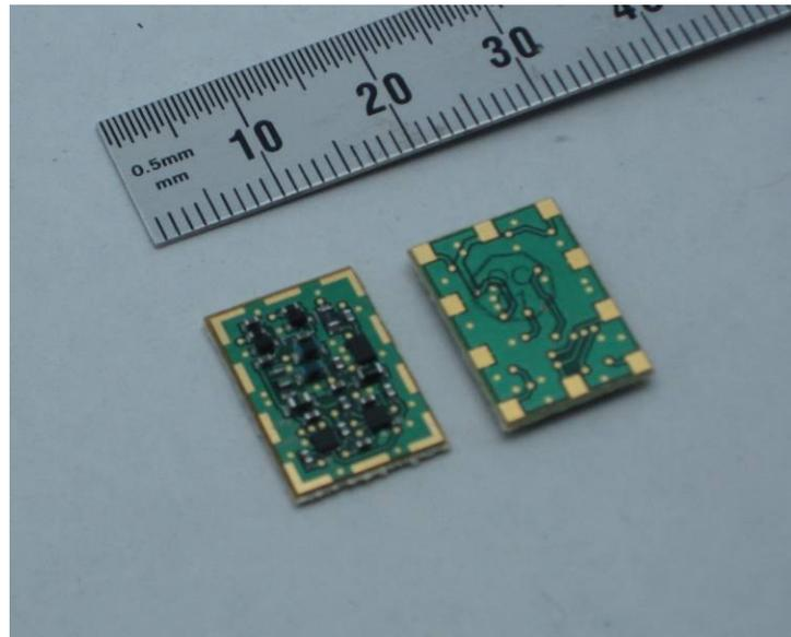
Figure 4. FASTROAD prototype module; top (left) and bottom (right) sides of module are shown
