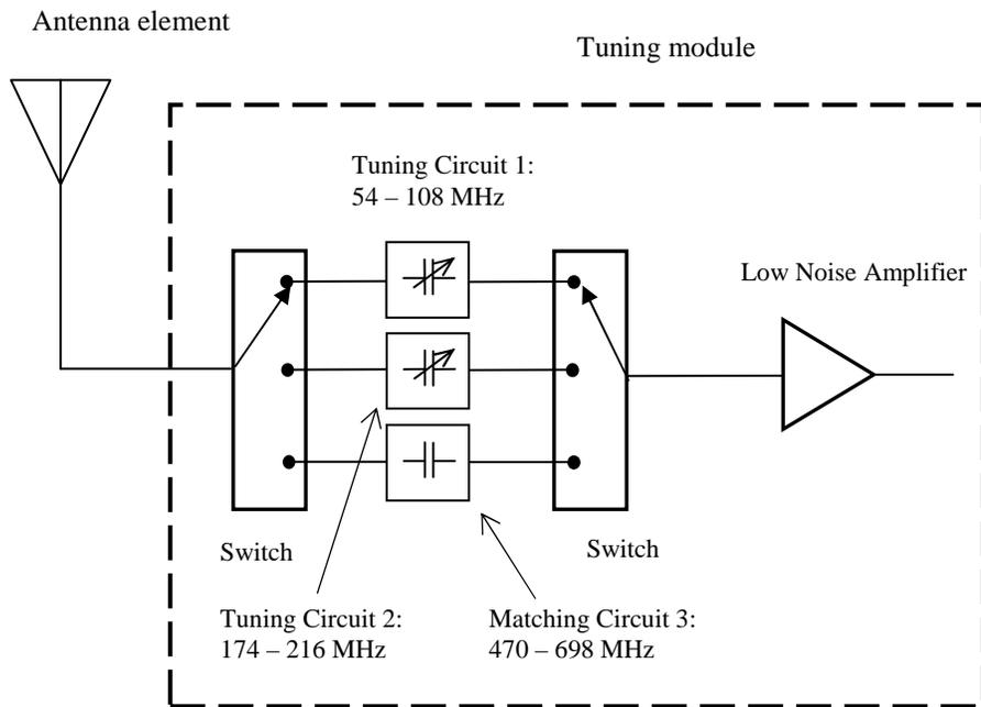
Figure 1. NAB FASTROAD embedded antenna topology
