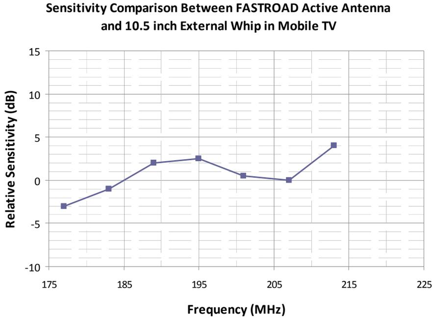
Figure 35. Measured comparison receiver sensitivity at VHF2
