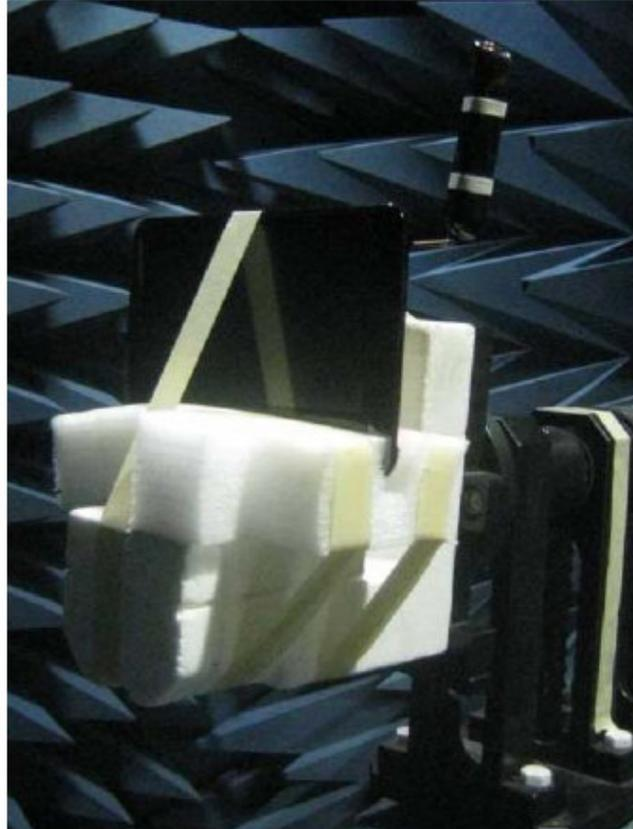
Figure 31. Modified mobile TV in anechoic chamber during test
