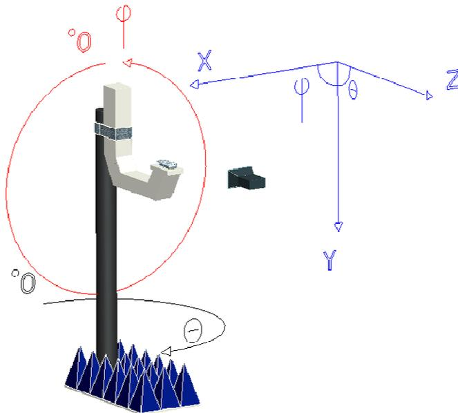
Figure 17. Coordinate system for all radiation pattern measurements, VHF1, VHF2, and UHF
