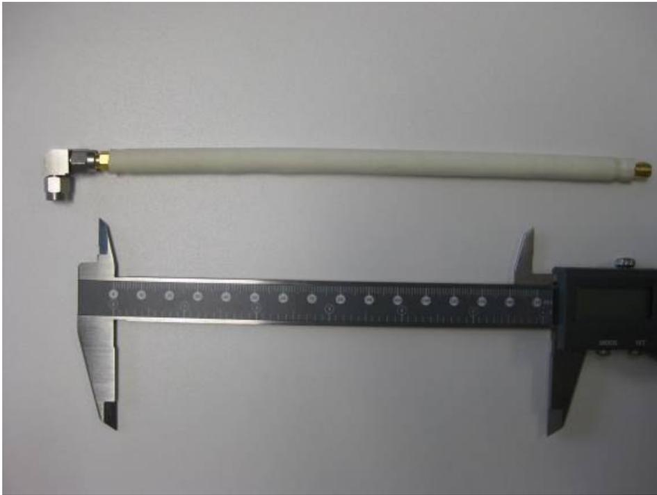
Figure 11. Ferrite loaded choke
