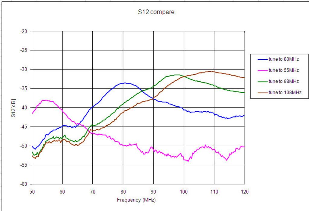
Figure 7. Tuning data for the VHF1 tuning circuit in the FASTROAD module
