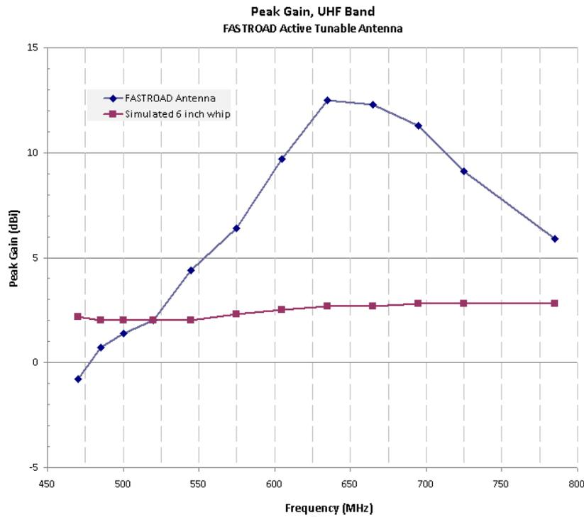
Figure 20. Measured peak gain of FASTROAD active tunable antenna at UHF band compared to simulated peak gain of 6 inch external whip antenna
