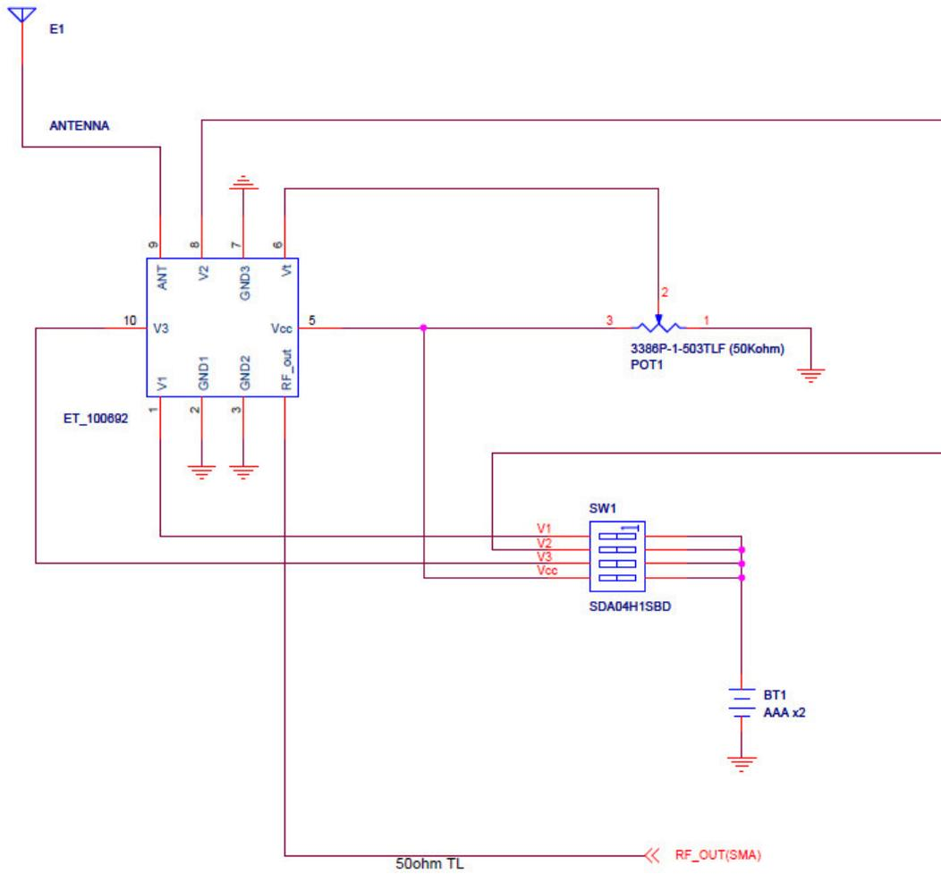
Figure 3. Control schematic for FASTROAD active tunable module
