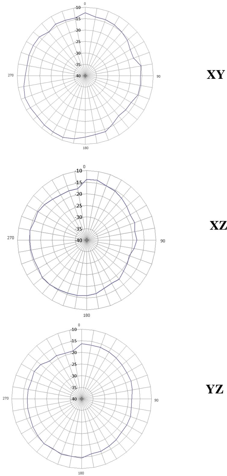
Figure 42. 2D radiation patterns at 196 MHz; scale is in dBi
