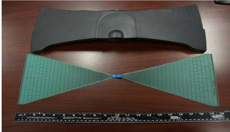
Figure 1-1: MegaWave 54-806 MHz Set Top TV Antenna, 1995
