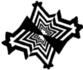
Figure 9 Wideband Dipole (Bowtie) by Fractenna
