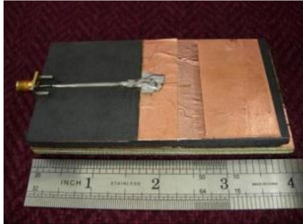
Figure 7: Lab Prototype of Wideband Dipole on EBG Material
